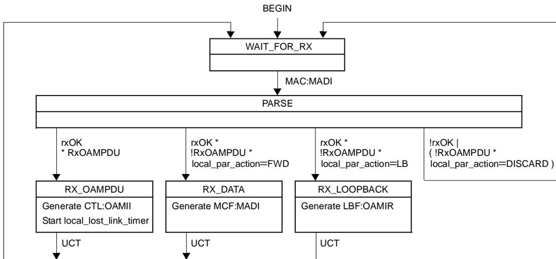
Figure 57–8—Parser state diagram
