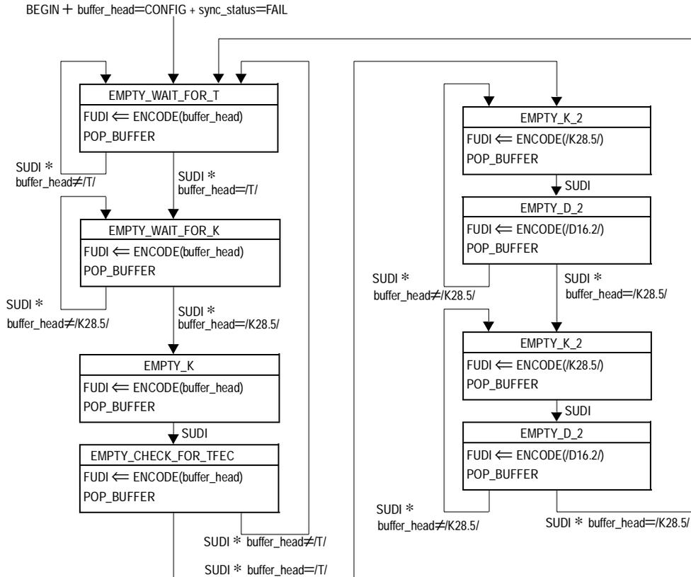
Figure 65–14—Receive buffer-empty state diagram
