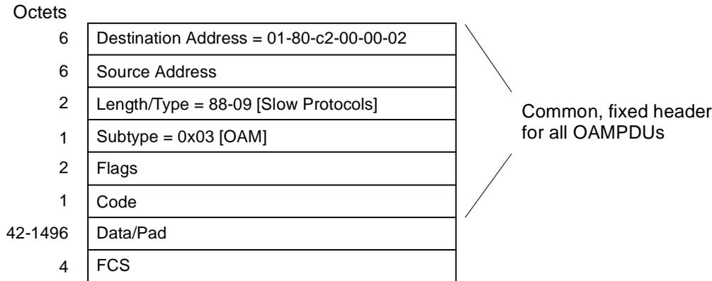
**Figure 57–9—OAMPDU frame structure**
