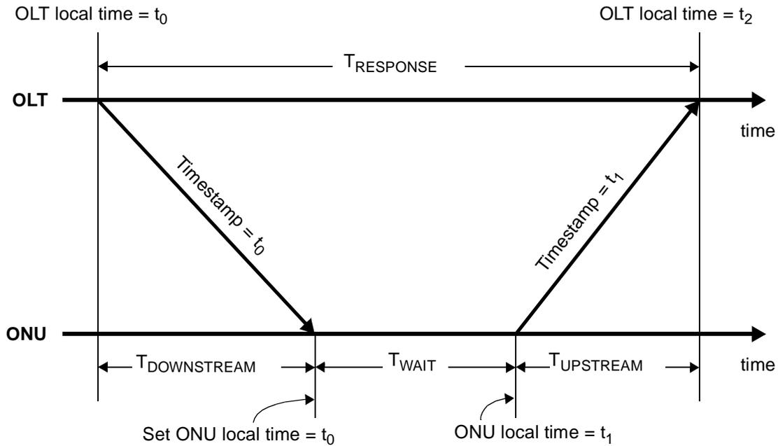
$T_{\text{DOWNSTREAM}}$  = downstream propagation delay
