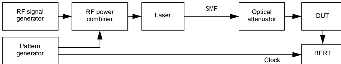
**Figure 59–6—Test setup for receiver bandwidth measurement**
