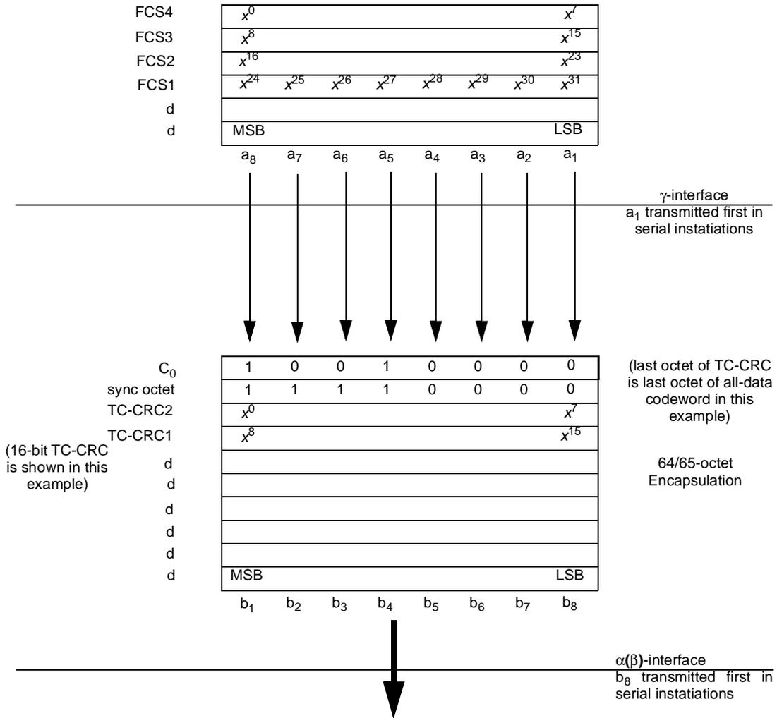
Figure 61-16— $\gamma$ -interface to  $\alpha(\beta)$ -interface bit ordering
