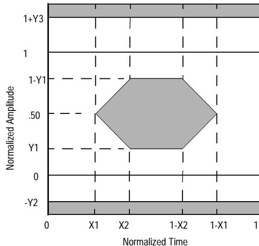
Figure 60–6—Transmitter eye mask definition
