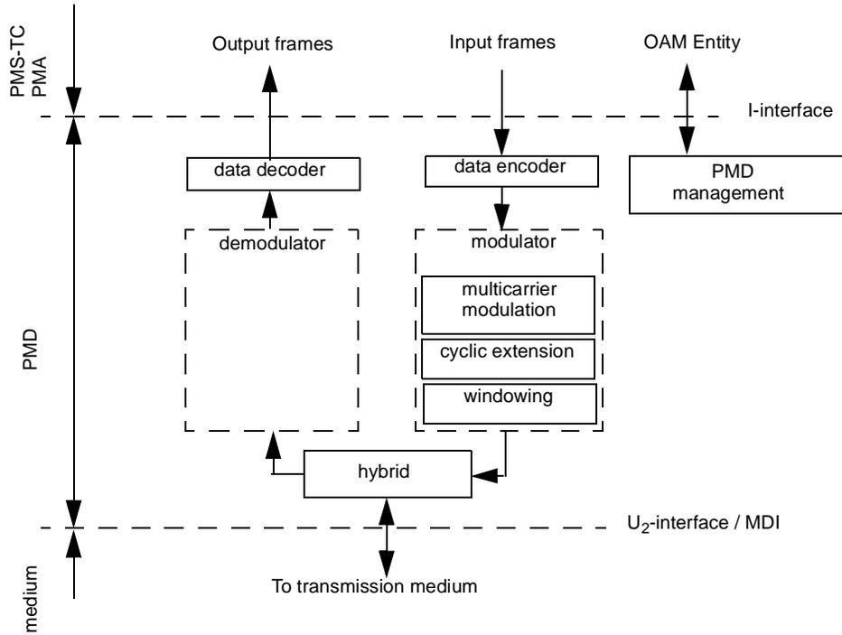
**Figure 62–2—Functional diagram of PMD sublayer**
