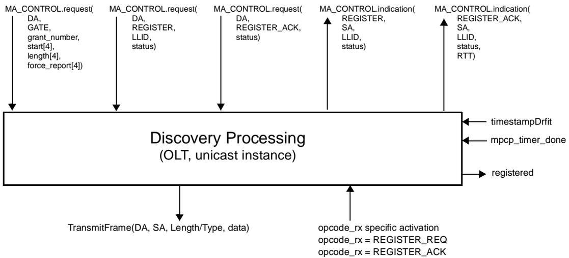
**Figure 64–16—Discovery Processing Service Interfaces (OLT, unicast instance)**
