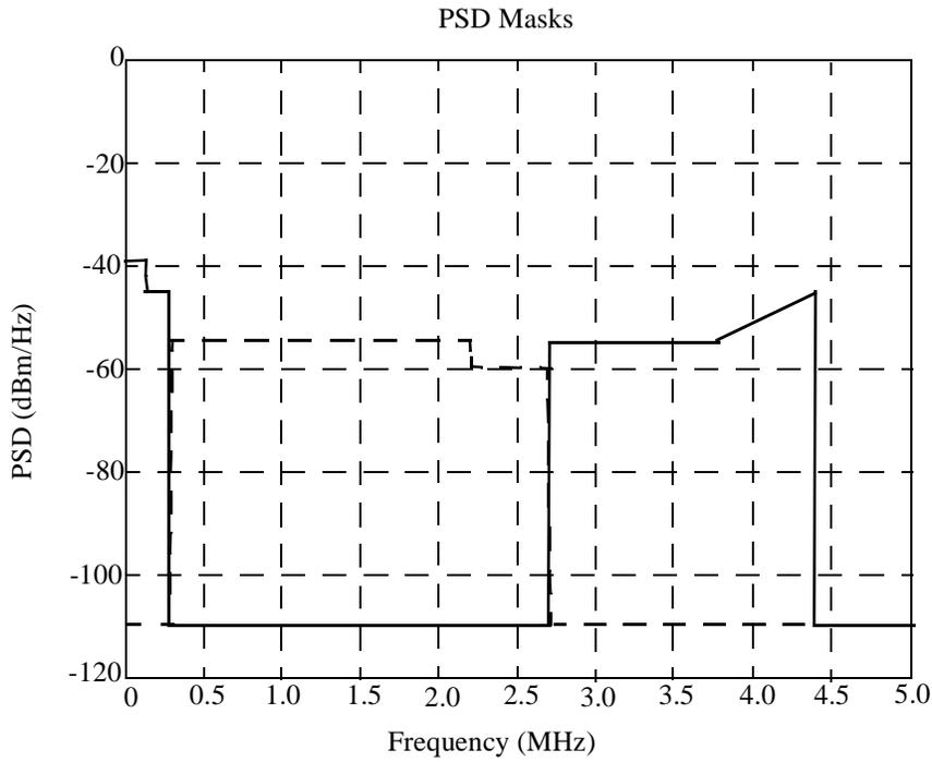
**Figure 62C-1—Example PSD Masks for MCM 10PASS-TS**
