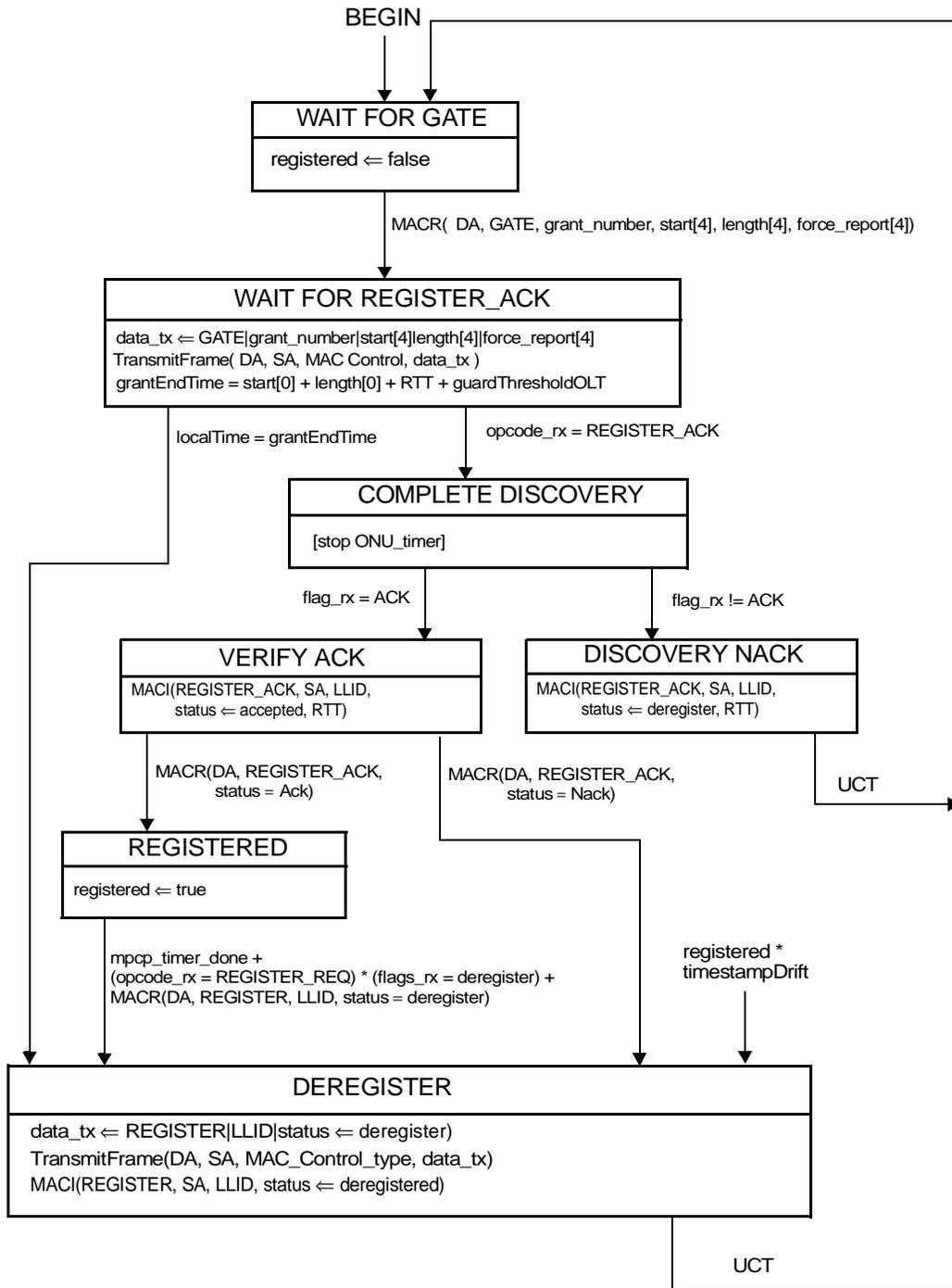
NOTE— The MAC Control Client issues the grant following the REGISTER message, taking the ONU processing delay of REGISTER message into consideration.
