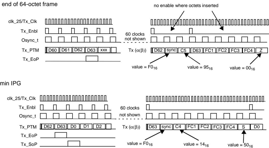
**Figure 61-14—Example transmit timing**
